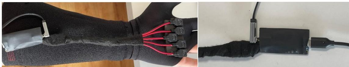
The foam wrap can be used to protect the board further and if required Velcro can be attached to it to secure in place. The board will power on automatically when connected to USB power source.
